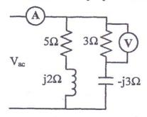
Q6. (A) Find current through  $5\Omega$  from A to B using Thevenin's theorem.
